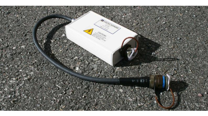
The LLD-702 is a long line driver for GSSI SIR® ground penetrating radar systems with low drive capacity. Radar systems such as the SIR3000 can drive cables with lengths up to 30 meters only, but with the aid of the LLD-702 cables in excess of 100 meters can be safely operated.
