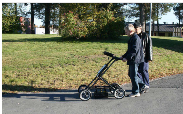
2. High resolution encoder is mounted on the standard cart without modifications.
