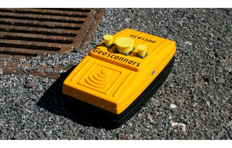
GCB-1500 expands the Geoscanners micrwoave frequency antennas. The purpose of this antenna is to be able to define small structures in concrete at shallow depths without compromising the penetration of it. It is possible to do rebars mapping, central heating pipes mapping, ice thickness in winter roads, as well as asphalt thickness measurements in surveys where the antenna can be in contact with the road.
