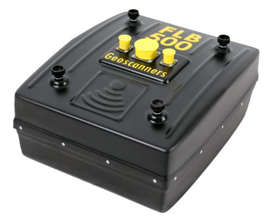
FLB-500 is an air launched ground penetrating antenna developed by Geoscanners AB to cover the need for noncontact survey applications. It has a narrow footprint on the air to ground interface to increase the amount of signal energy penetrating into the ground. FLB-500 has been optimized to offer a good front to back ratio allowing operation in urban environment as well.
