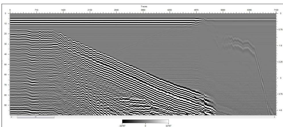
2. Air to water transition during the antenna calibration.
