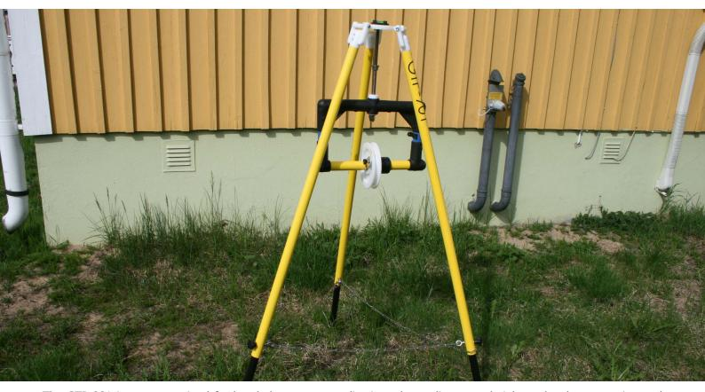
The GTP-901 is a survey tripod for borehole antenna applications demanding extra height under the measuring and cable feeding pulley. The tripod has an integrated GSSI compatible encoder unit to facilitate the distance mode in borehole applications. The unit is made of strong materials such as fiber glass reinforced pipes and POM milled parts.
