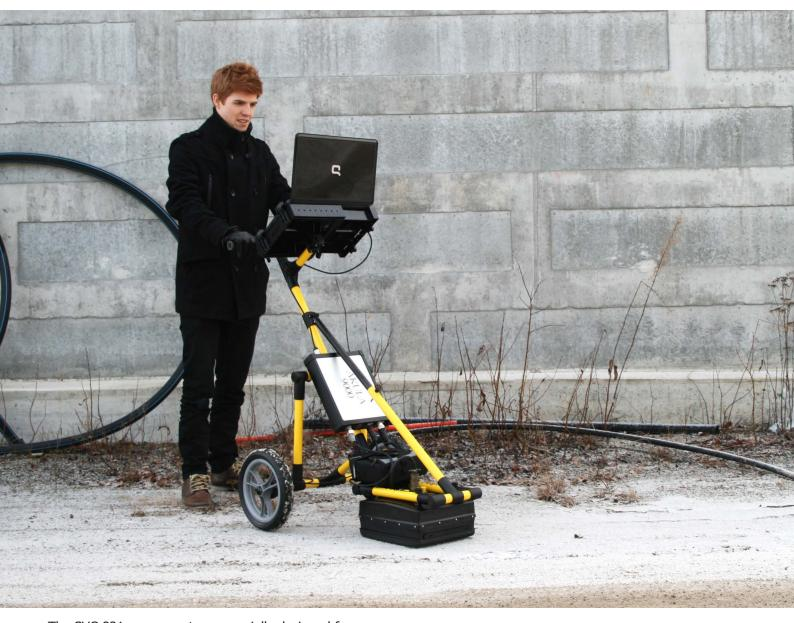
The SVC-821 survey cart was specially designed for the U-Explorer Mini system based on the radar control units from the Akula 9000 series, as well as ground coupled antenna from the GCB-series (200MHz-700MHz).
