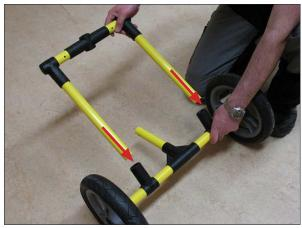
3. Insert the angle adjuster (4) into the lobger yellow pipe of the main frame (5).
