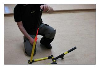
4. Connect the main frame (5) to the back axis(1).
