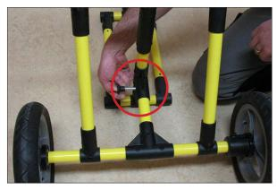
6. Insert the handle (4) through the back frame (2) into the main frame (5).
