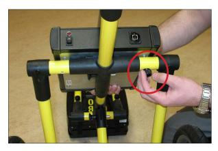
4. The survey cart is now assembled. Now only the control cable, USB cable and the encoder need to be conected to complete the radar configuration.
