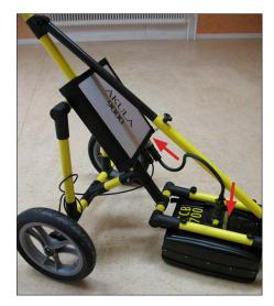
6. After connecting the control cable you are ready to install the battery in the rear top part of the antenna, where the plastic hinges of the frame are located.
