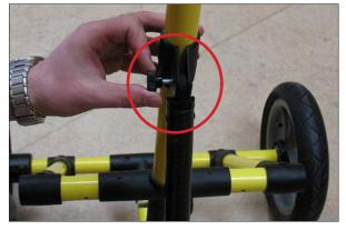
8. Use a quick release pin (7) to fit one of the two available holes on the angle adjuster (4) to set the prefered angle of the main frame (5) to the antenna.
