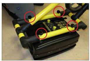
3. With the supplied thumbscrews (8) secure your radar control unit Akula 9000 to the back frame. Please note that the On/Off button and the USB output need to face up.
