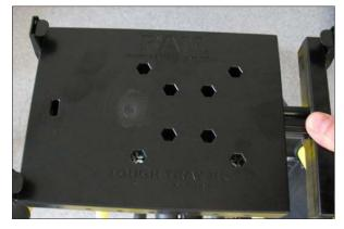
5. Hold the control unit with one hand and insert the fixing thumb screws from behind the horizontal bars. Continue with the rest of the thumb screws until the control unit is secured in place.
