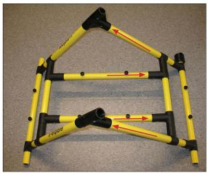
3. Insert the quick release bolts with the red button into the holes to secure the connections.
