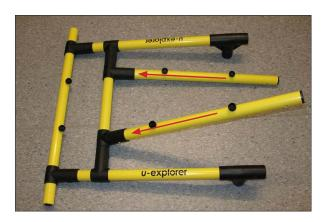
2. Use the assembled piece from the previous step and connect it to the back end of the cart. Push simultaneously the antenna holder pipes into the slots on the back end of the cart and the back end pipes into the T junction slots.
