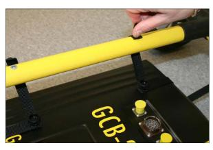
4. Place the computer delivered with the GPR system into the computer plate holder. Make sure that the spring latch mechanism has a good grip on the computer and that the quick snap clip is tightened enough to hold the computer when mounted.
