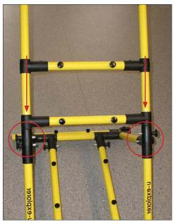
5. Find the wheel with the encoding ring on it and insert it into the socket where the encoder is located. Insert the rest of the wheels afterwards.
