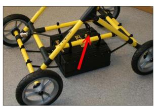
8. Connect the other end of the control cable from step 7 to the control unit.
