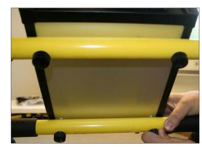
6. Put the battery pack on the back axle and fasten the two belts around the back axle and the horizontal bar as shown in the picture.
