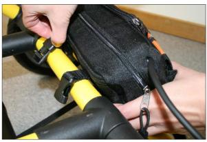
7. Connect the main control cable to the antenna using the green metal connector side of the cable.
