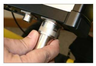
9. Connect the supplied survey wheel cable to the encoder
