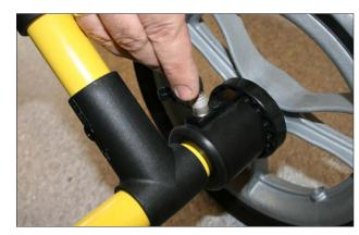
10. Connect the other end of the survey wheel cable from step 9 to the radar control unit.
