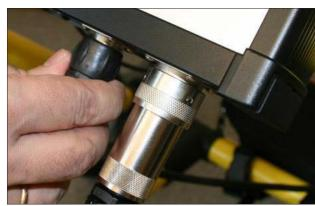
11. Connect the power cable to the control unit and secure it with the lock.
