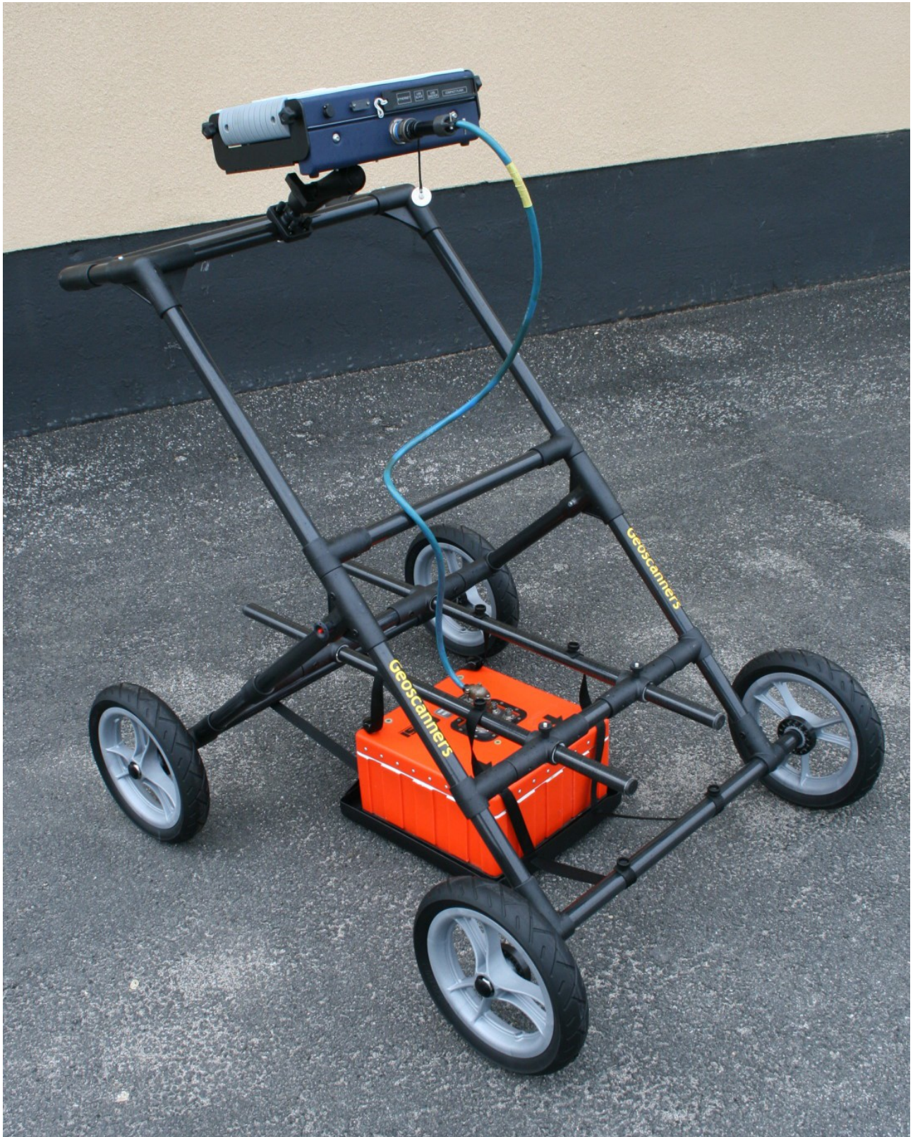
Final view of the survey wheel cart SVC-819 with the SVC81950400ADP mounted.
