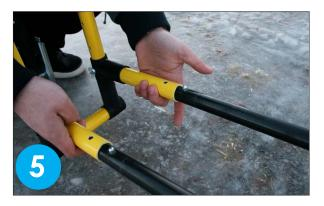
Repeat steps 3-4 to insert the black pipes into the front frame of GST-806.
