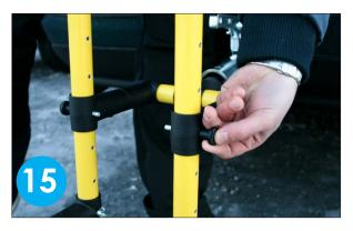
Use quick release bolts to adjust the height of the vehicle mount and antenna.
