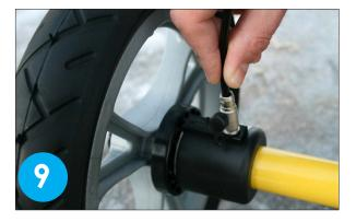
Connect one end of the survey wheel encoder cable to your ENC-820 survey wheel encoder.
