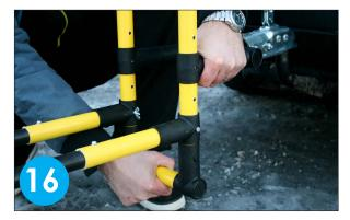
Adjust the front height of the GST-806 vehicle mount by sliding the front frame up or down to different pre-drilled positions.
