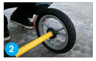
Insert the wheel without the magnetic ring on the other side of the back frame.
