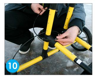
Always wrap the cable around one of the pipes of the back frame. This minimizes the chance of breaking the cable.
