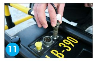
Connect the survey wheel encoder cable to your antenna.
