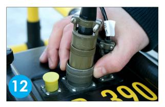
Connect the provided control cable to your antenna.
