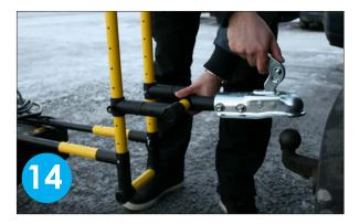
Connect the provided hook to your vehicle. Make sure that it is secured.
