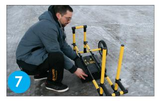
Use the screws to secure your antenna. The antenna should be oriented so that the labels are readable from the front side of the vehicle mount.
