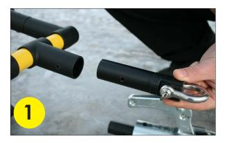
Remove the standard car hook from the front frame and insert the snow mobile extension as shown above.
