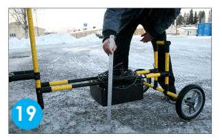
Make sure that the height adjustments position the antenna as parallel to the ground as possible. This is done to ensure a good quality of your data collection.
