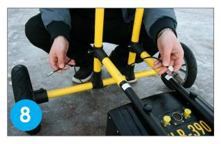
Connect the survey wheel cable once your antenna is in place.
