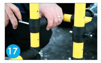
Use the pre-drilled holes and quick-release bolts to secure the position of the front frame.
