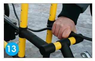
Secure the control cable at the front of the vehicle mount. Allow for enough slack so that the cable is not stretched. Make sure that it is not hanging close to the ground neither.
