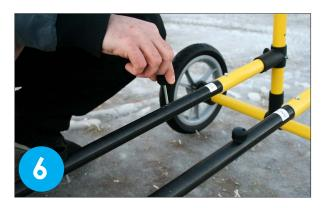
Insert the provided antenna screws.
