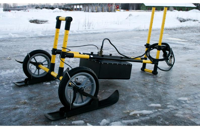
GST-806 is a vehicle mounted antenna holder, designed for high speed GPR surveys. Its height is easily adjusted to fit different vehicles.
