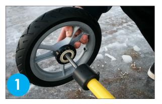
Insert the wheel with the magnetic ring to the back frame as shown above.
