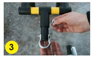
Secure the snow mobile extension by using the provided wingnut for your locking screw.
