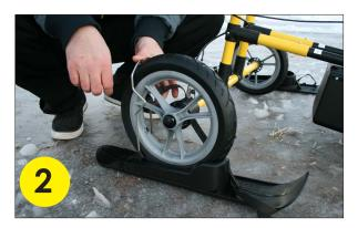
Lift the metal fixture so that it presses the wheel.
