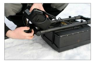
4. Connect the survey wheel cable to the encoder.
