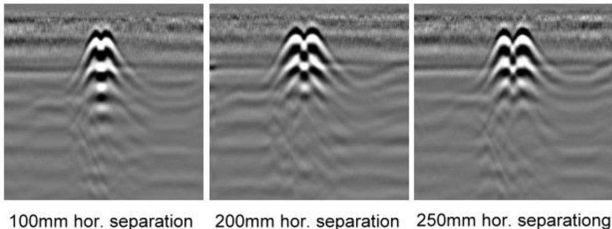
*Fig. 7 Experiments results for the horizontal resolution separation*
