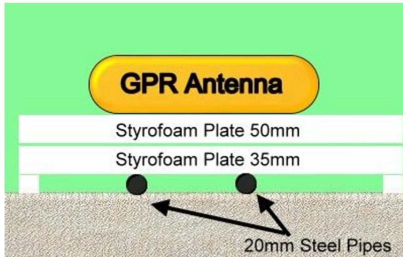
*Fig. 6 Setup for the horizontal resolution experiment.*
