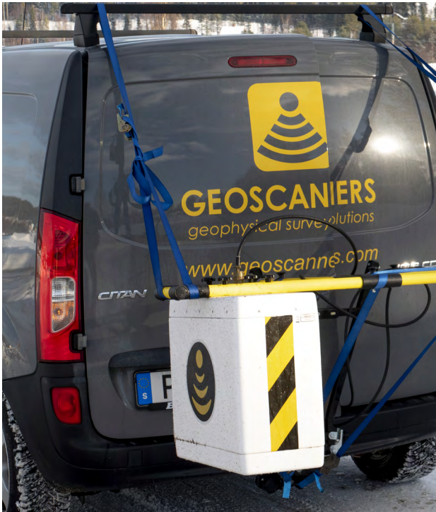
1. The antenna is easily mounted on a vehicle.
